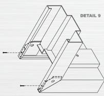
Secure or save glass bead for installation of glass and glazing
