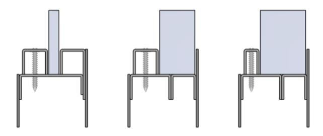
5/8" Glazing bead and reinforcement channels are all 16GA
